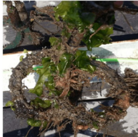
Figure 17. UWPT coil bottom after 45 days [115].
