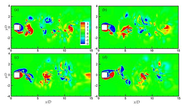
**Figure 13.** Instantaneous contours of the spanwise vorticity  $\omega_z$  for  $\alpha = 15^\circ$  on the (x, y) plane at z = 4D within one vortex shedding period T. (a) t = 0; (b) t = T/4; (c) t = 2T/4; (d) t = 3T/4.
