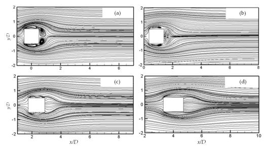
**Figure 11.** Time-averaged streamlines for different yaw angles viewed on the (x, y) plane at z = 4D. (a)  $\alpha = 0^{\circ}$ ; (b)  $\alpha = 15^{\circ}$ ; (c)  $\alpha = 30^{\circ}$ ; (d)  $\alpha = 45^{\circ}$ .
