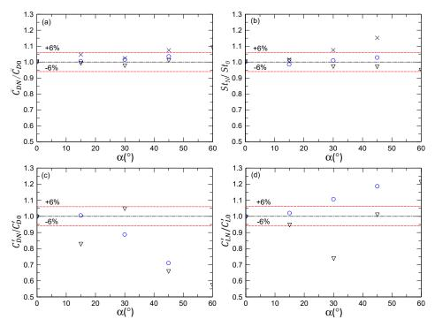
**Figure 7.** Ratios of force coefficients and Strouhal number at various cylinder yaw angles with those at  $\alpha = 0^{\circ}$ . (a)  $\overline{C}_{DN}/\overline{C}_{D0}$ ; (b)  $St_N/St_0$ ; (c)  $C'_{DN}/C'_{D0}$ ; (d)  $C'_{LN}/C'_{L0}$ . The dashed lines denote  $\pm 6\%$  tolerances. The dash–dotted lines denote a ratio of 1.  $\bigcirc$ : Present study, square cylinder;  $\times$ : Lou et al. [19], square cylinder;  $\nabla$ : Zhao et al. [10], circular cylinder.
