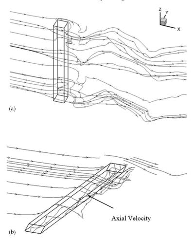
**Figure 18.** Streamlines around the cylinder for different yaw angles. (a)  $\alpha = 0^{\circ}$ ; (b)  $\alpha = 45^{\circ}$ .
