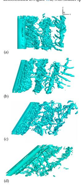
**Figure 10.** Instantaneous iso-surfaces of  $\lambda_2$  for different yaw angles at the same phase ( $\lambda_2 = -1$ ). (a)  $\alpha = 0^\circ$ ; (b)  $\alpha = 15^\circ$ ; (c)  $\alpha = 30^\circ$ ; (d)  $\alpha = 45^\circ$ .
