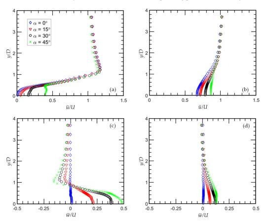
**Figure 5.** Time-averaged profiles of the streamwise  $(\overline{u}/U)$  and spanwise  $(\overline{w}/U)$  velocity for different yaw angles at two downstream locations. (**a**,**c**) x = 1D; (**b**,**d**) x = 10D.
