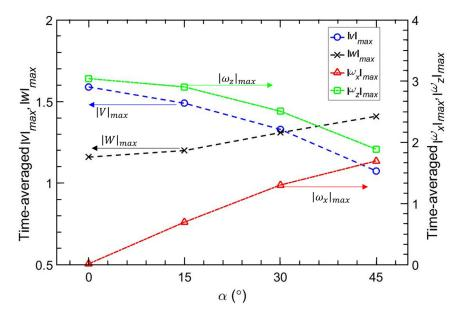
Figure 17. Variations of the time-averaged maximum velocity and vorticity for different yaw angles.
