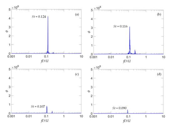
**Figure 6.** Energy spectra of the lift coefficient for different cylinder yaw angles. (a)  $\alpha = 0^{\circ}$ ; (b)  $\alpha = 15^{\circ}$ ; (c)  $\alpha = 30^{\circ}$ ; (d)  $\alpha = 45^{\circ}$ .
