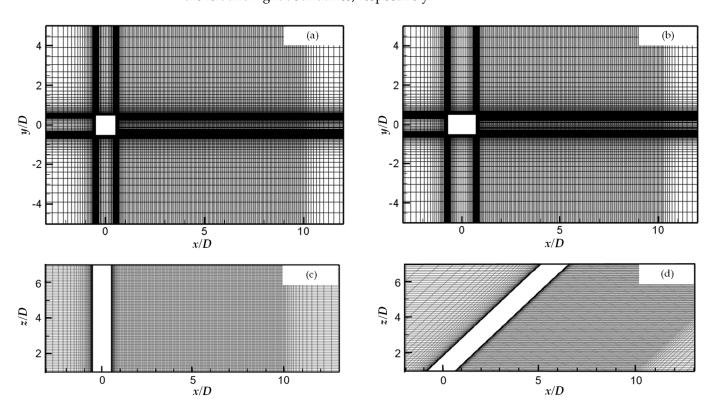
**Figure 2.** A close-up view of the mesh. Top view on plane z=0: (a)  $\alpha=0^\circ$ ; (b)  $\alpha=45^\circ$ . Side view on plane y=0: (c)  $\alpha=0^\circ$ ; (d)  $\alpha=45^\circ$ .
