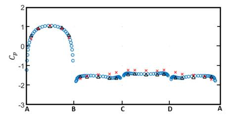
**Figure 8.** Distributions and comparison with previous studies of the time-averaged pressure coefficient on the cylinder surfaces for  $\alpha = 0^{\circ}$ .  $\bigcirc$ : Present study, Re = 1000;  $\triangle$ : Norberg [35], Re = 5000;  $\times$ : Sohankar et al. [16], Re = 500.
