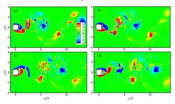
**Figure 12.** Instantaneous contours of the spanwise vorticity  $\omega_z$  for  $\alpha = 0^\circ$  on the (x, y) plane at z = 4D within one vortex shedding period T. (a) t = 0; (b) t = T/4; (c) t = 2T/4; (d) t = 3T/4.
