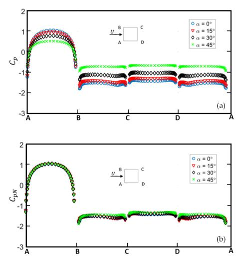
**Figure 9.** Distributions of the time-averaged pressure coefficient on cylinder surfaces for different yaw angles. (a) Calculated using the freestream velocity U; (b) calculated using the freestream velocity component normal to the cylinder axis  $U_N$ .
