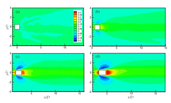
**Figure 16.** Contours of the time-averaged spanwise velocity w for different yaw angles viewed on the (x, y) plane at z = 4D. (a)  $\alpha = 0^\circ$ ; (b)  $\alpha = 15^\circ$ ; (c)  $\alpha = 30^\circ$ ; (d)  $\alpha = 45^\circ$ .
