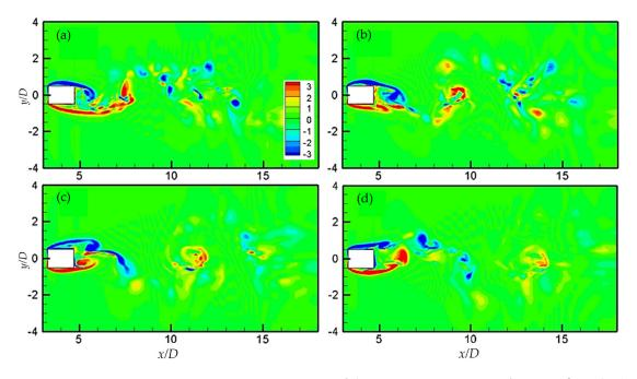
**Figure 15.** Instantaneous contours of the spanwise vorticity  $\omega_z$  for  $\alpha = 45^\circ$  on the (x, y) plane at z = 4D within one vortex shedding period T. (a) t = 0; (b) t = T/4; (c) t = 2T/4; (d) t = 3T/4.
