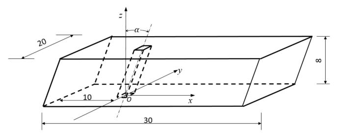
**Figure 1.** Schematic diagram of the coordinate and the computational domain (unit in *D*).
