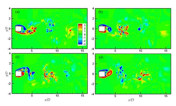
**Figure 14.** Instantaneous contours of the spanwise vorticity  $\omega_z$  for  $\alpha = 30^\circ$  on the (x, y) plane at z = 4D within one vortex shedding period T. (a) t = 0; (b) t = T/4; (c) t = 2T/4; (d) t = 3T/4.
