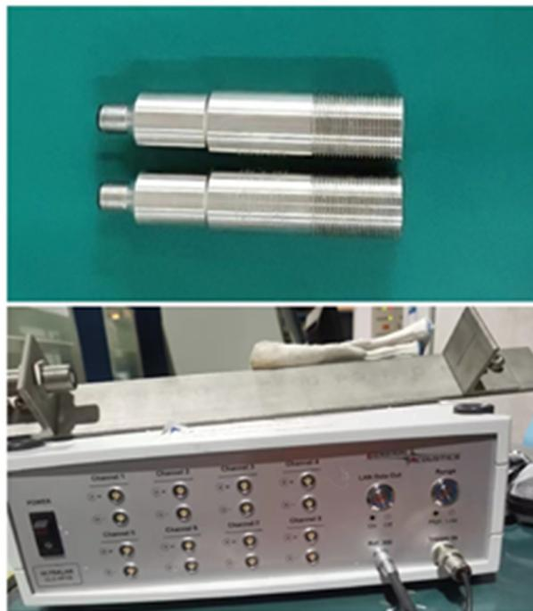
**Figure 4.** Wave gauges (top) and its acquisition system (bottom).
