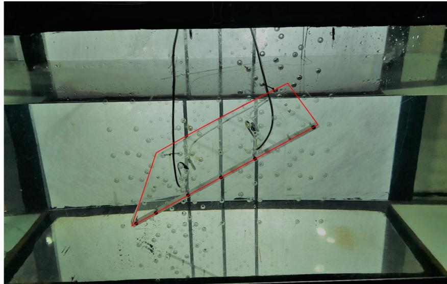
**Figure 3.** The inclined submerged plate in the experiment which is highlighted by the red line.
