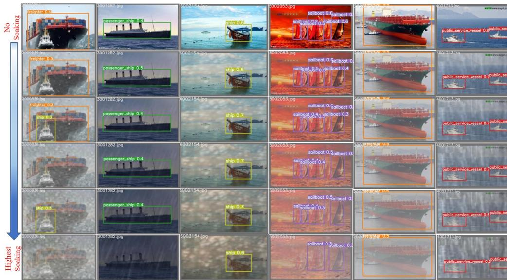
**Figure 17.** The performance of FRSD at different soaking degrees. Each column of pictures shows the detection results under different rain and fog scenes.
