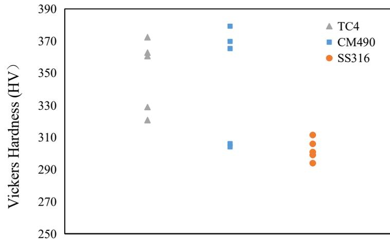
**Figure 6.** Test results of the Vickers hardness.
