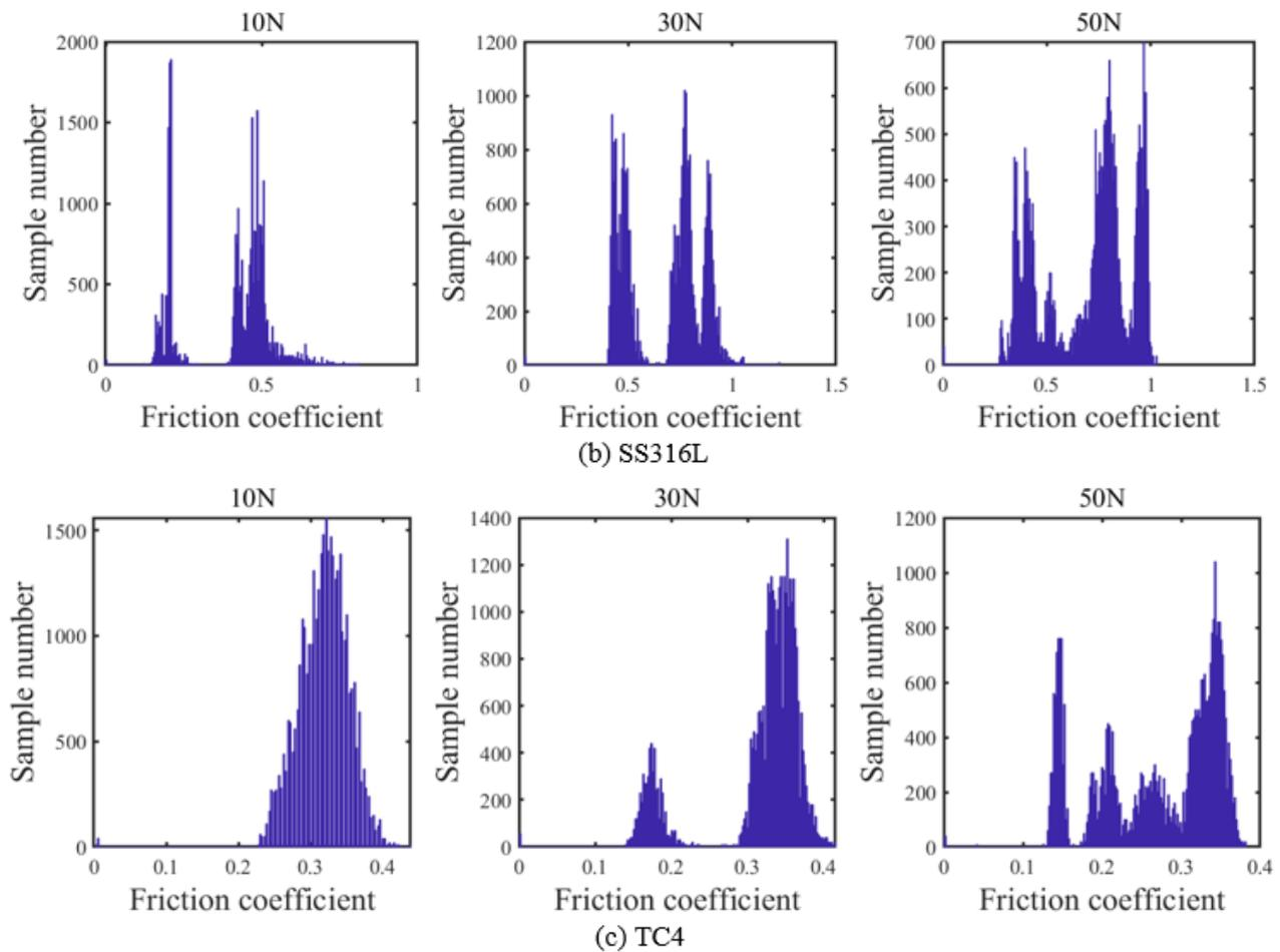
Figure 10. Statistical graphs of friction coefficients at each test condition.
