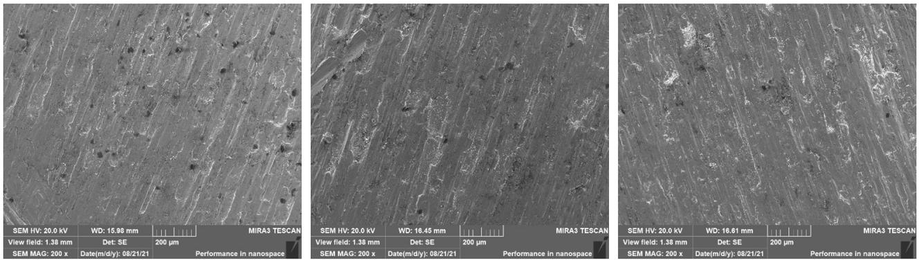
(b) CM490 ( $F = 10, 30, \text{ and } 50 \text{ N}$ ), pin specimen
