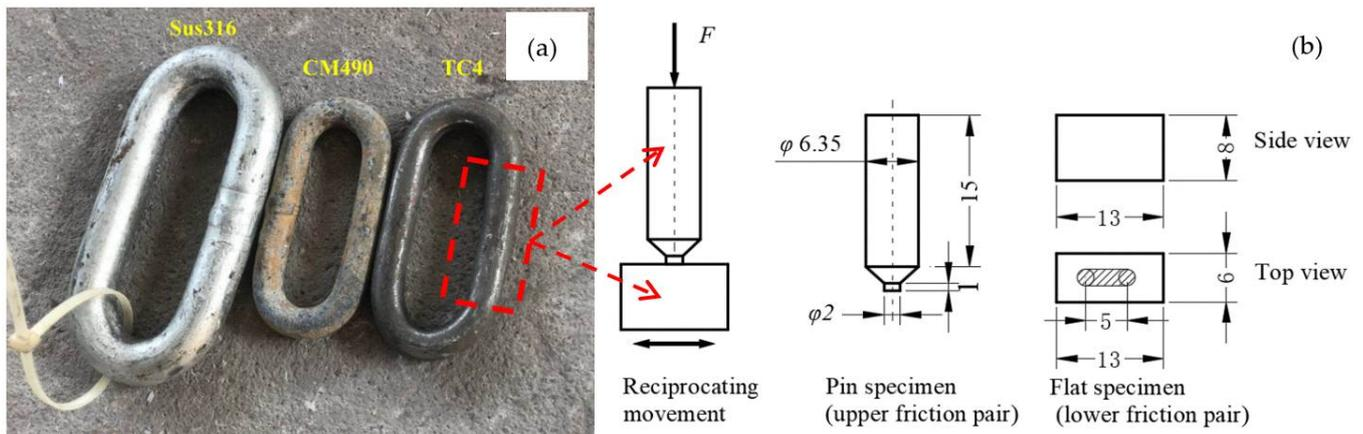
Figure 5. (a) Chains links formed of different materials and (b) pin-on-flat friction pair.
