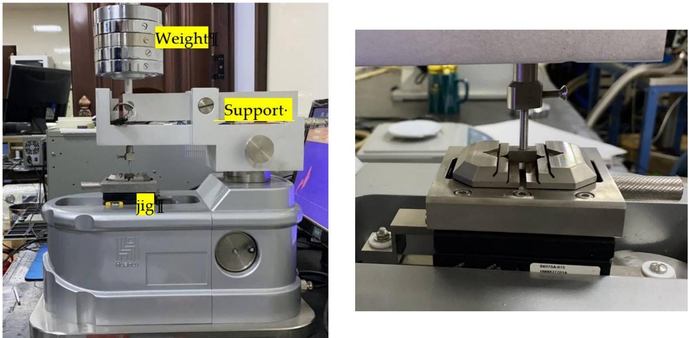
Figure 4. MFT-R4000 high speed reciprocating friction and wear tester (Lanzhou Institute of Chemical Physics, China).
