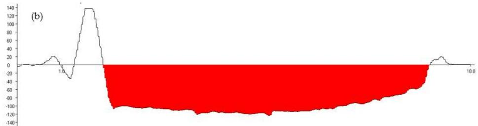
**Figure 3.** Wear depth measurement (Unit:  $\mu\text{m}$ ) (a): along the width direction (b): along the wear direction.
