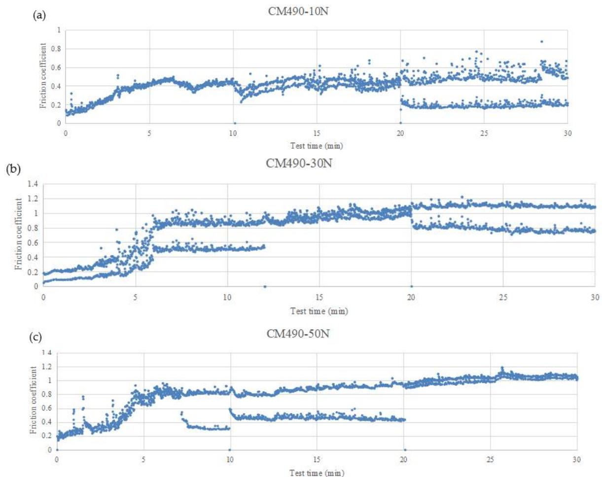
**Figure 7.** Friction coefficient of CM490 as a function of test time. (a)  $F = 10$  N (b)  $F = 30$  N (c)  $F = 50$  N.
