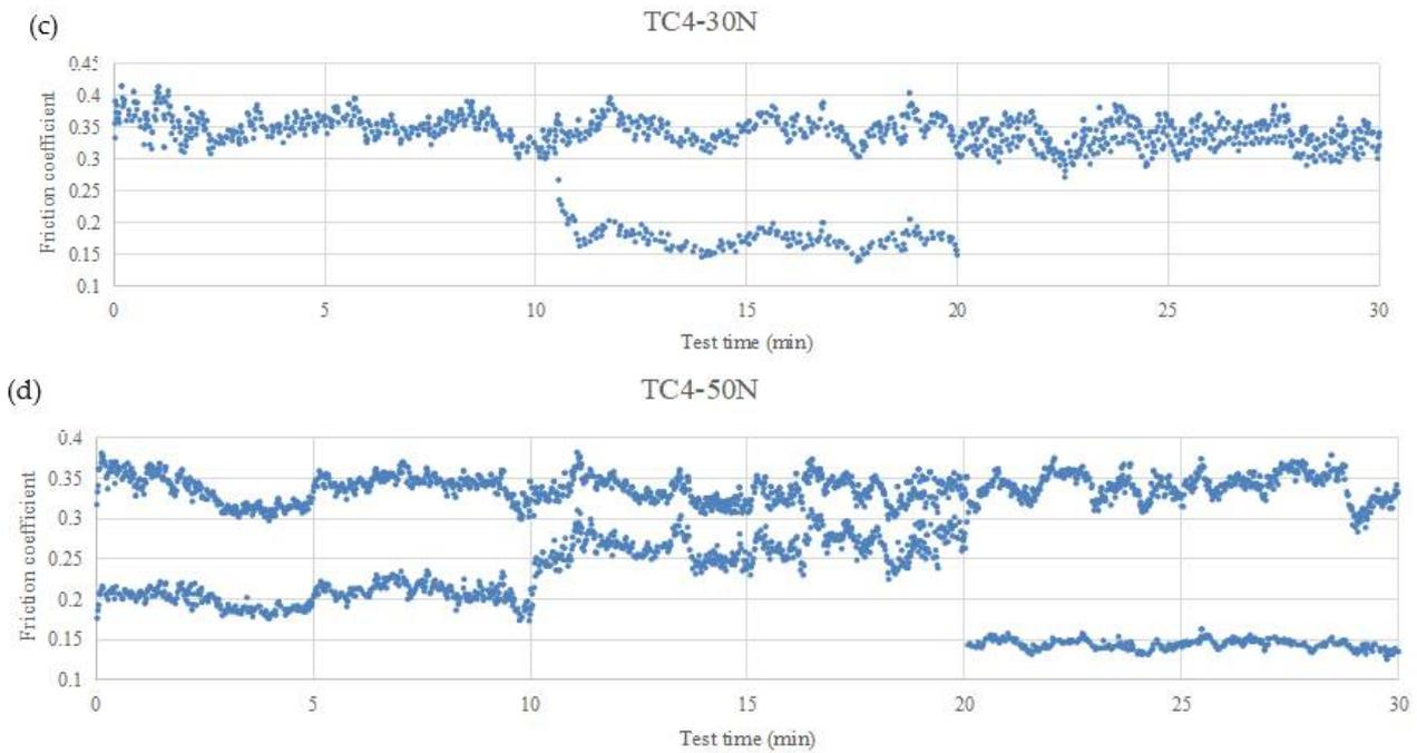
**Figure 9.** Friction coefficient of TC4 as a function of test time (a)  $F = 10\text{ N}$  (c)  $F = 30\text{ N}$  (d)  $F = 50\text{ N}$  (Note: the time scales in (b-1,b-2) are different, where a single sample point can be clearly observed in (b-2)).
