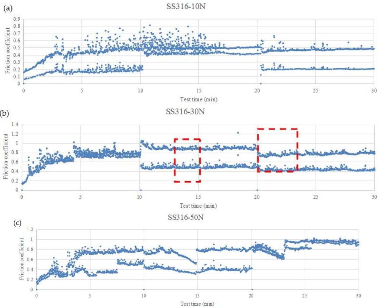
Figure 8. Friction coefficient of SS316 as a function of test time. (a)  $F = 10\text{ N}$  (b)  $F = 30\text{ N}$  (c)  $F = 50\text{ N}$ .
