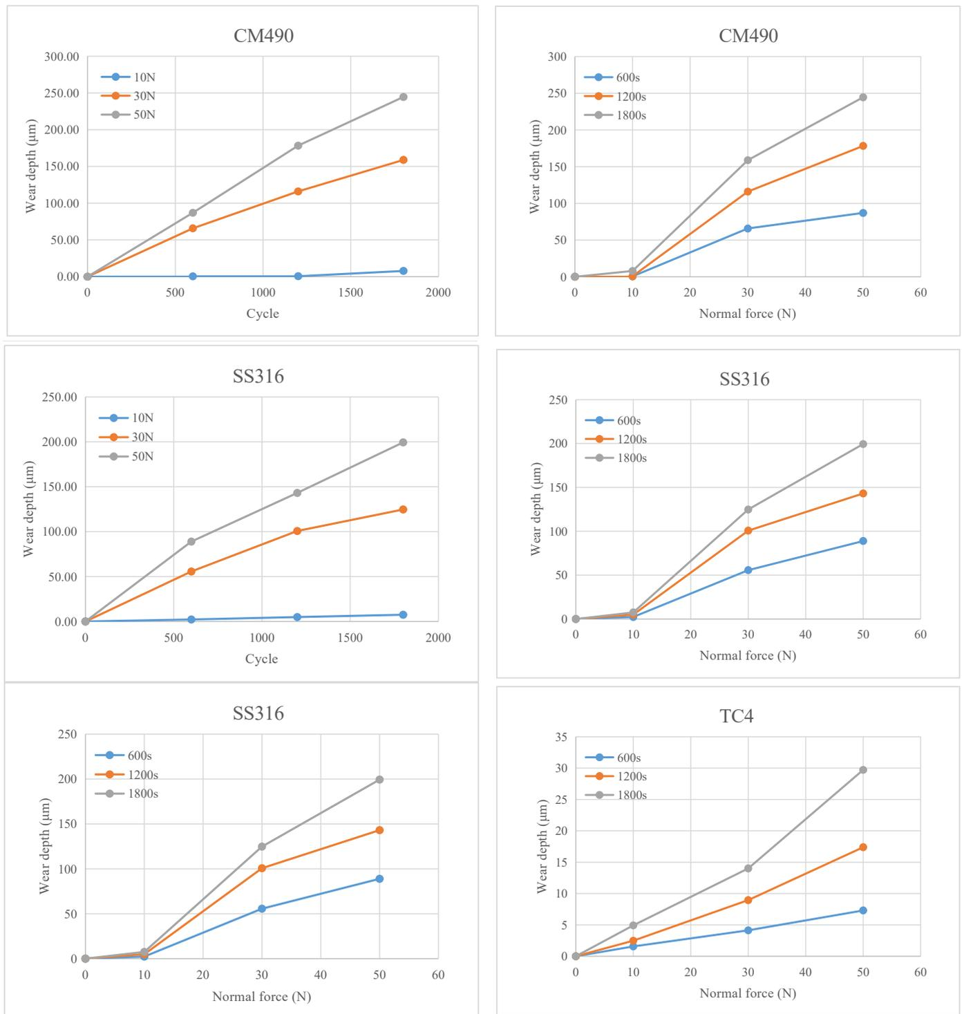
Figure 13. Wear depth as a function of wear cycle and applied normal force.
