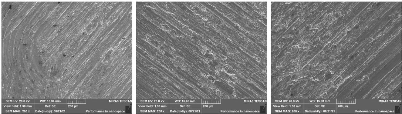
(f) TC4 ( $F = 10, 30, \text{ and } 50 \text{ N}$ ), pin specimen
