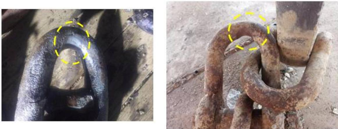
**Figure 1.** Typical wear pattern of chain links in the contact region (recovered from buoys in South China Sea).
