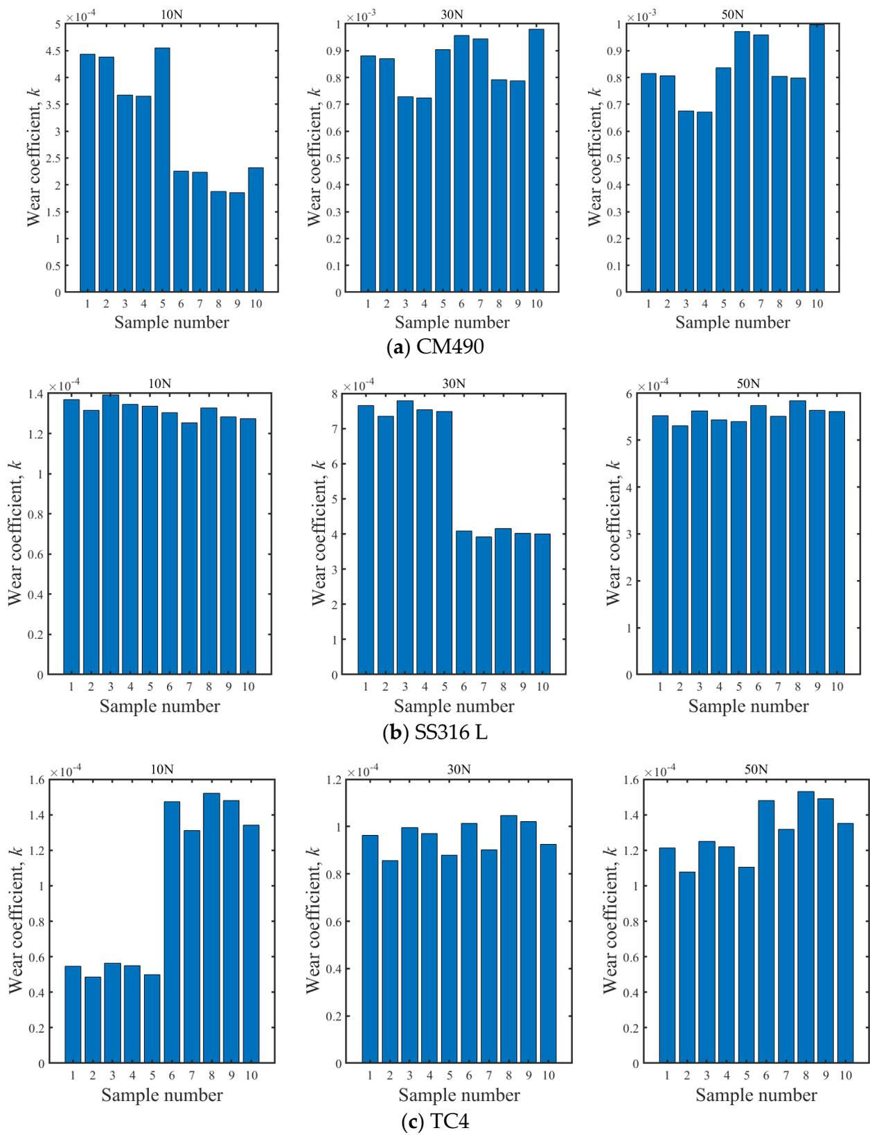
**Figure 14.** The variability of wear coefficient considering the variation of hardness (The second and third stages).
