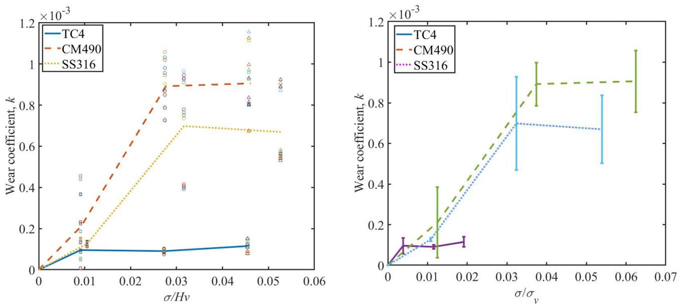
**Figure 15.** Wear coefficient as a function of contact stress to hardness ratio ( $\sigma/Hv$ ) and contact stress to yield stress ratio ( $\sigma/\sigma_y$ ) (the total error bar lengths are double the standard deviation values of the calculated wear coefficient).
