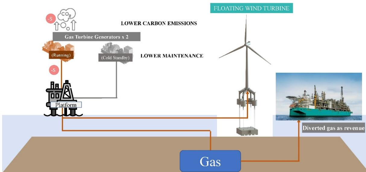
Figure 3. Hybrid power generation concept.
