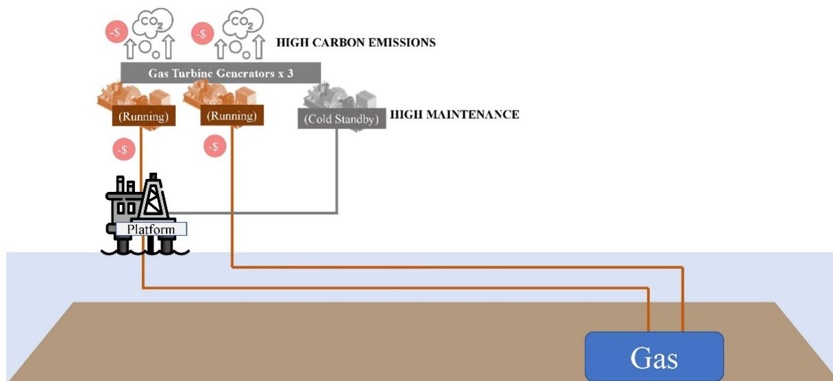
**Figure 1.** Conventional power generation concept.
