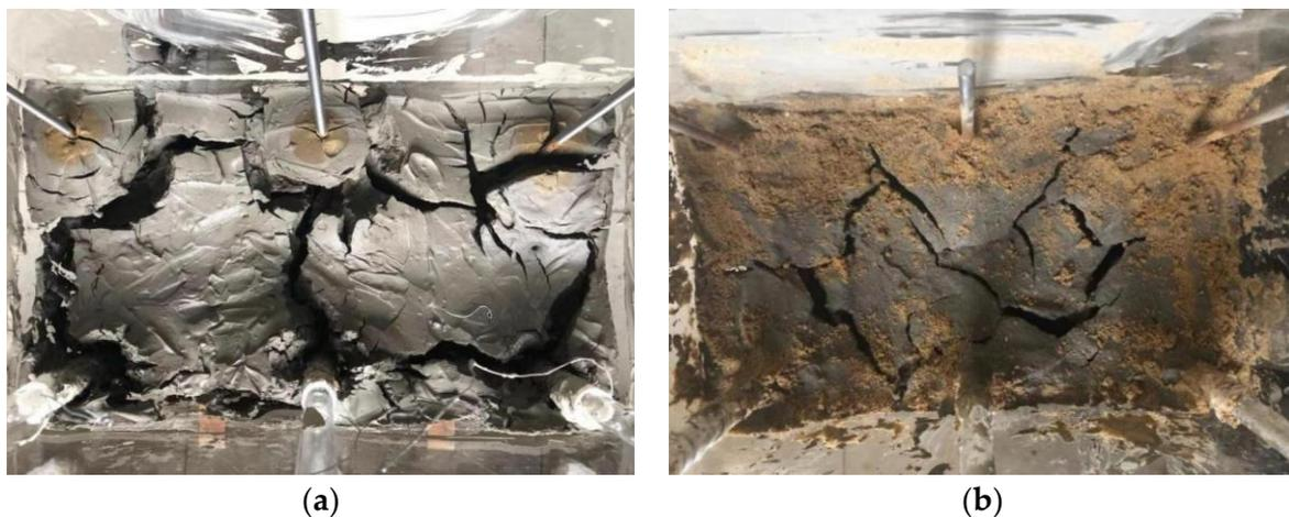
**Figure 5.** Soil cracks that developed during the tests: (a) The soil state after T1 test; (b) The soil state after T2 test.
