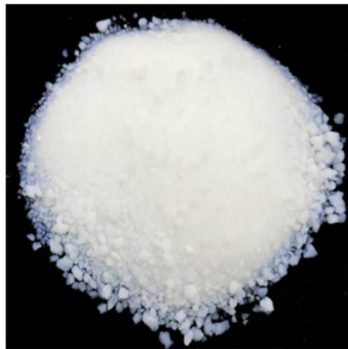
**Figure 4.** Photography of silica-based aerogels.
