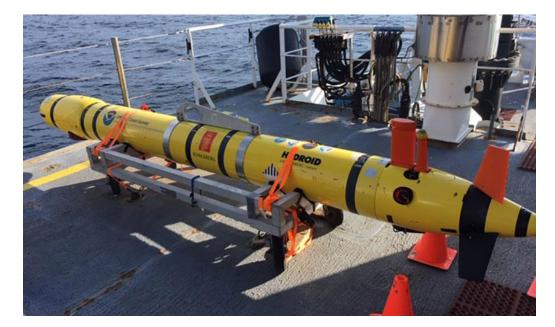
**Figure 2.** Remus 600 unmanned underwater vehicle used by the National Oceanic and Atmospheric Administration (NOAA) [4]. Image used is consistent with NOAA policy, "NOAA still images, audio files and video generally are not copyrighted. You may use this material for educational or informational purposes, including photo collections, textbooks, public exhibits, computer graphical simulations and webpages." [3].
