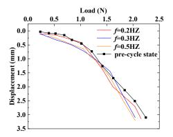
Figure 8. Load displacement curves with different cyclic frequencies.
