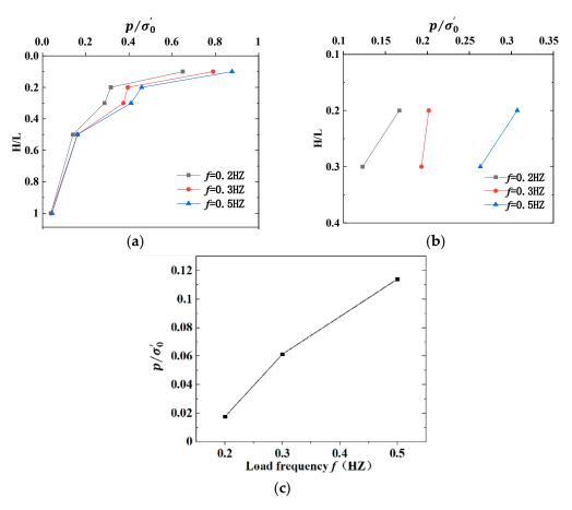
**Figure 3.** Normalized pore water pressures with different cyclic load frequencies: (**a**) close to the wall; (**b**) 0.8 D from the wall; (**c**) 1.2 D from the wall (at 0.2 L).
