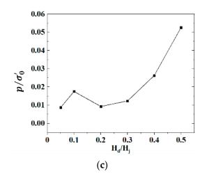
**Figure 2.** Normalized pore pressures with different horizontal cyclic load amplitudes: (**a**) close to the wall; (**b**) 0.8 D from the bucket; (**c**) 1.2 D from the bucket(0.2 L).
