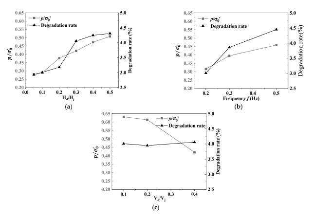
**Figure 5.** Relationship between  $p/\sigma'_0$  and undrained shear strength degradation rate: (**a**) horizontal cyclic load amplitude ratio; (**b**) horizonal cyclic load frequency; (**c**) vertical load ratio.
