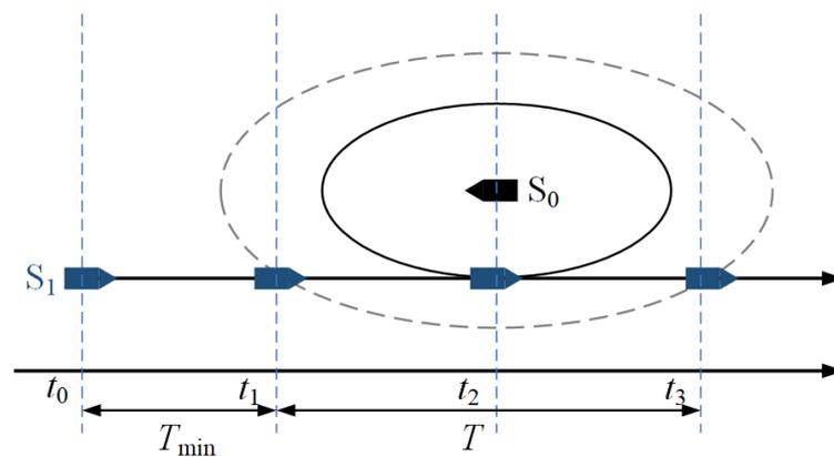
Figure 7. Schematic diagram of collision risk parameters.
