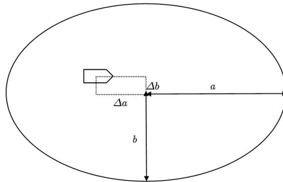
**Figure 4.** A decentralized elliptic ship domain.
