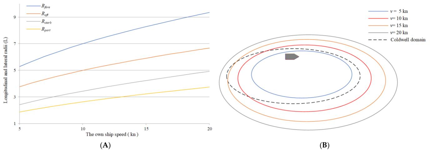
**Figure 6.** (A) The radii of the elliptical dynamic ship domain for various ship speeds; (B) combined elliptical dynamic ship domain and Coldwell domain.
