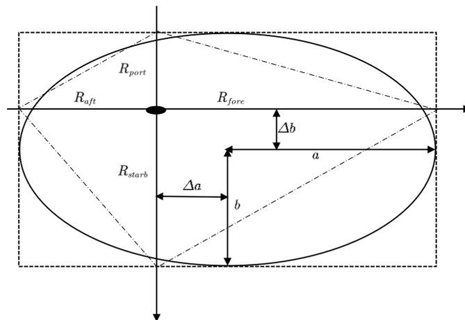
Figure 5. Elliptic dynamic ship domain model.
