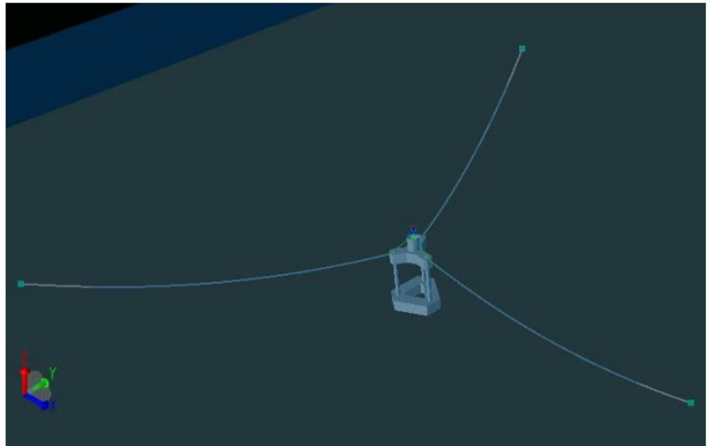
**Figure 3.** Coupled model in SESAM DeepC<sup>®</sup>.
