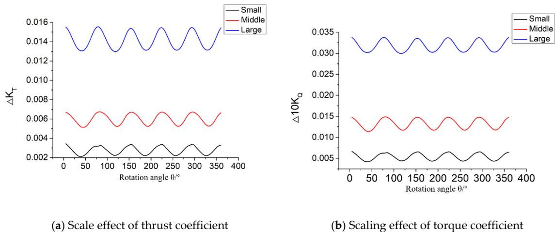
**Figure 22.** Fluid–structure coupling scale effect of composite propeller.
