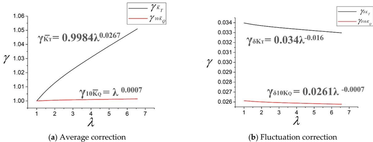
Figure 15. Scaling effect correction of unsteady hydrodynamic coefficients for rigid propeller.
