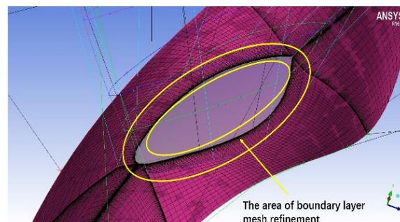
**Figure 3.** Boundary layer grid.
