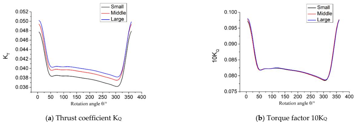
Figure 12. Periodic variation of unsteady force of a single rigid blade.
