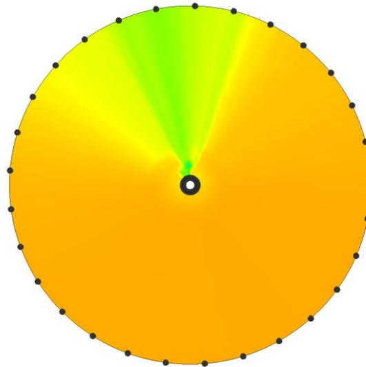
**Figure 4.** Inlet velocity contour of non-uniform wake flow field.
