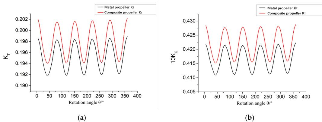
**Figure 21.** Comparison of the hydrodynamic performance of a small-scale composite propeller and a rigid propeller. (a) Thrust coefficient comparison during a rotation period. (b) Comparison of torque coefficients during a rotation period.
