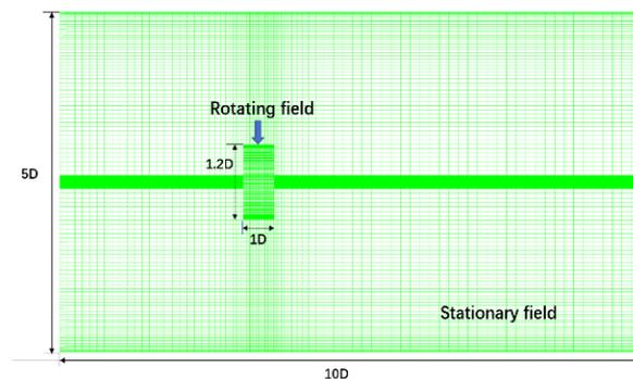
**Figure 2.** Rotating and stationary fluid domain.
