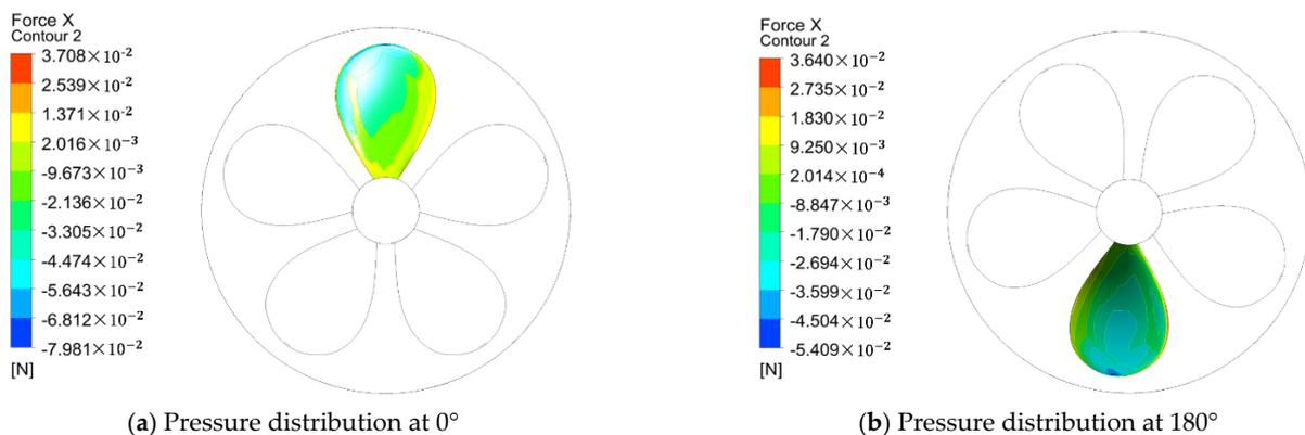
Figure 13. Pressure distribution of the blade through the low- and high-speed area.
