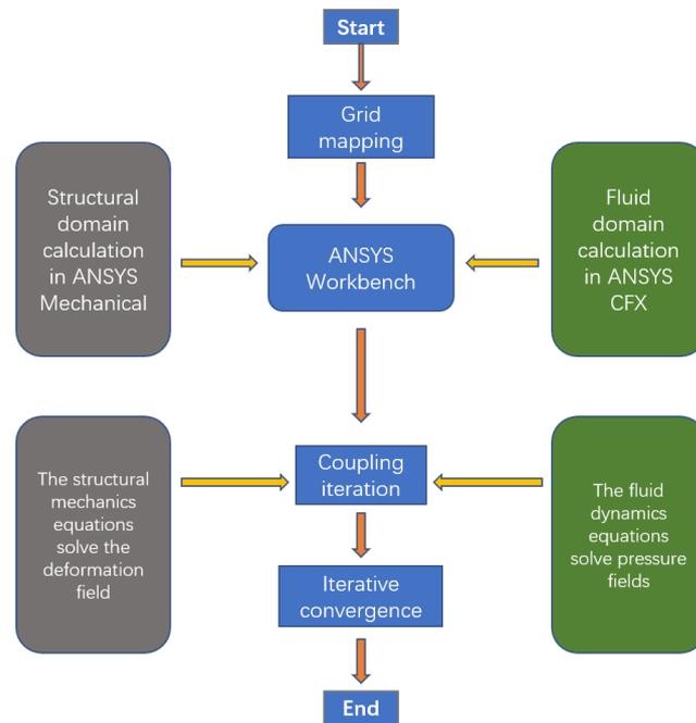
**Figure 1.** Solution work flow of fluid–structure coupling iterative method.
