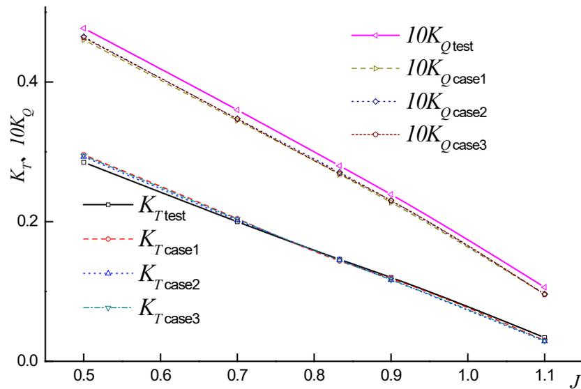
Figure 5. Comparison between experimental data and calculation values of the open water performance in three cases.
