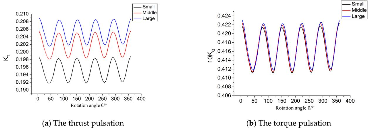
Figure 14. Unsteady hydrodynamic performance pulsation of rigid propeller.
