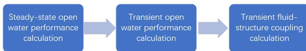
Figure 11. Flow chart of transient fluid–structure coupling calculation.
