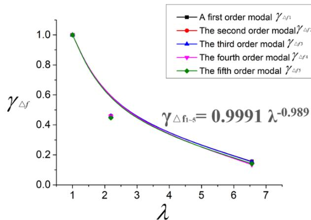
Figure 19. Correction of amplitude scaling effect of wet-mode natural frequency reduction.
