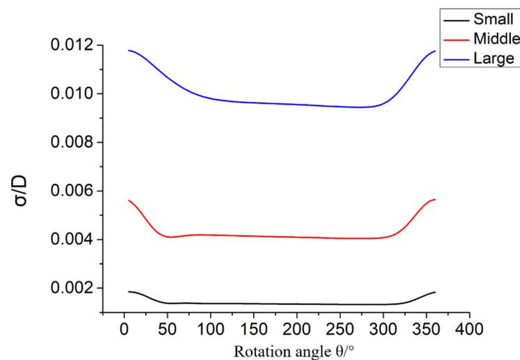
Figure 16. Maximum deformation ratio of a single propeller with different scales in a rotation period.
