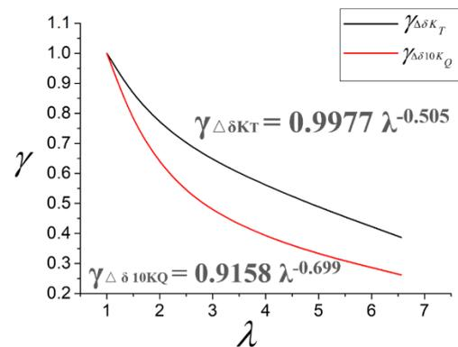
Figure 24. Scale effect correction of composite propeller’s unsteady force pulsation with different scales.
