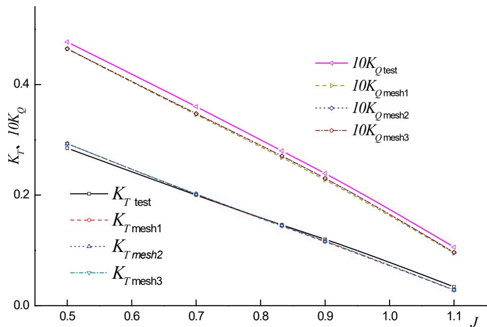
Figure 7. Comparison between experimental and calculated values of the open water performance with different grid numbers.
