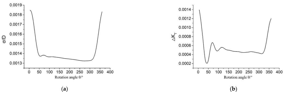
Figure 20. The corresponding relationship between the maximum deformation ratio and the thrust coefficient difference. (a) The maximum deformation ratio. (b) The thrust coefficient difference before and after fluid–structure coupling.
