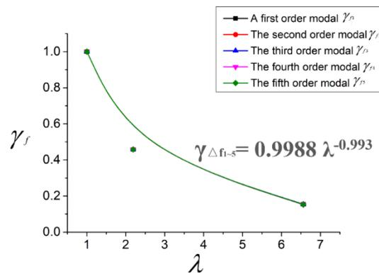
**Figure 18.** Scale effect correction of dry mode natural frequency with different scales.
