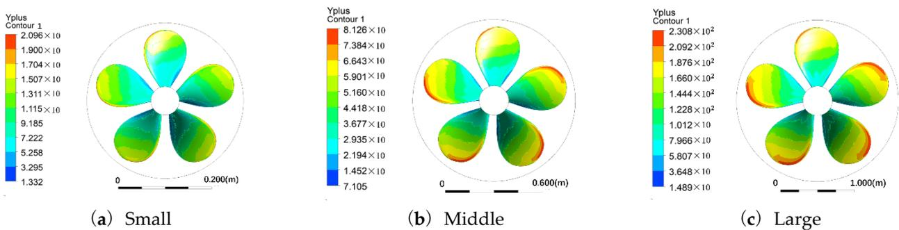
Figure 6.  $Y^+$  distribution at different scales.
