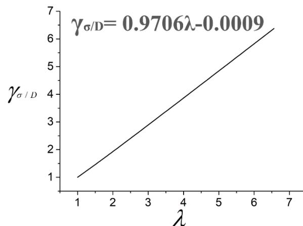
**Figure 17.** Maximum deformation ratio scale effect correction of composite propeller in transient fluid–structure coupling.
