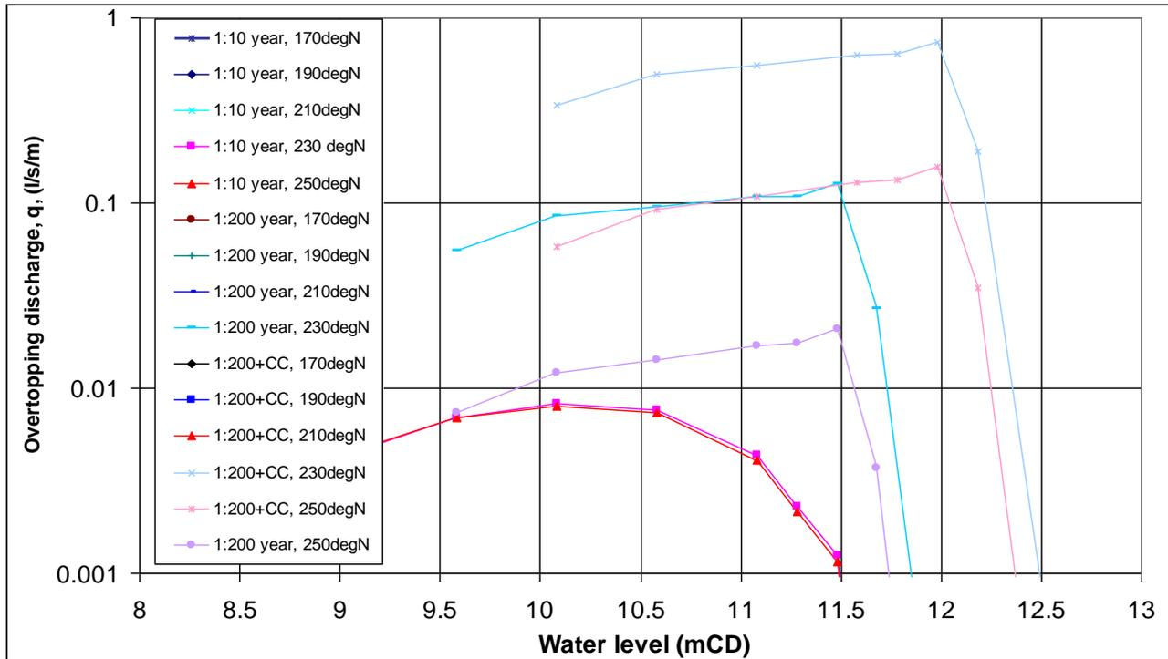
Figure 13. Overtopping at Position C1, wide crest at +19 mCD.
