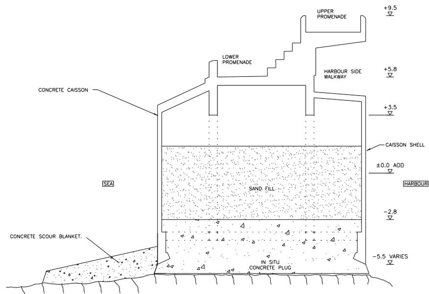
Figure 4. Example breakwater caisson.
