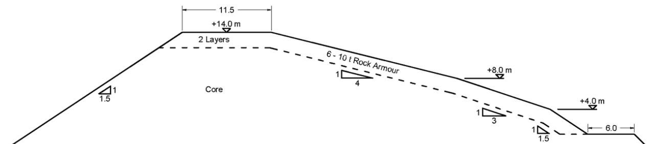
Figure 8. La Collette reclamation breakwater section, as model tested in 1993.
