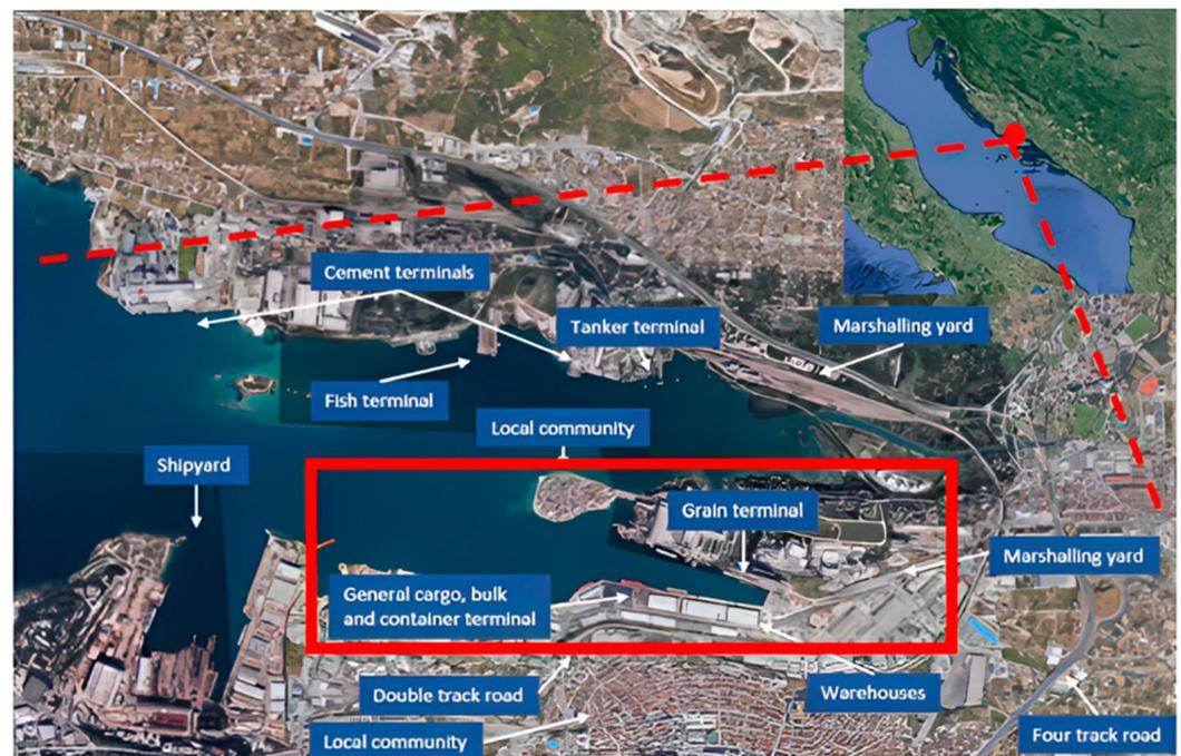
**Figure 2.** Overview of the cargo basin and infrastructure with indication of its functions ([46], modified).
