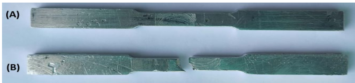
Figure 3. Samples used in the tensile test; (A) before and (B) after the test.
