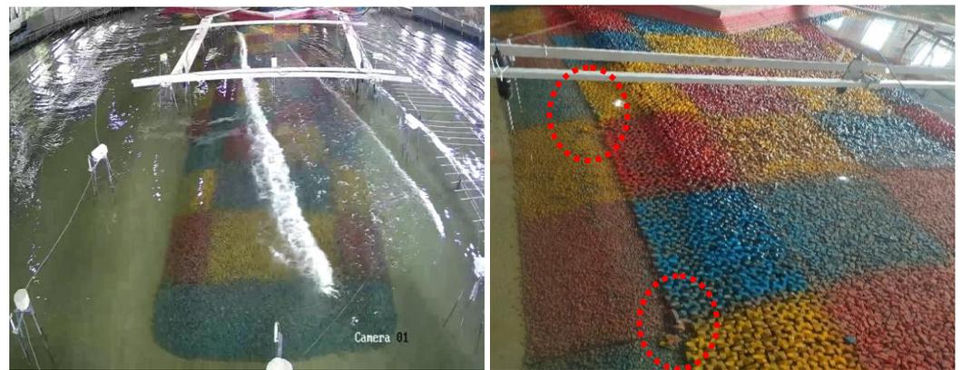
(a) Wave breaking along the overburden surface (b) Instability of 8 t Accropode at the toe of slope
