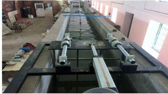
Figure 5. Wave flume and wave generator system.
