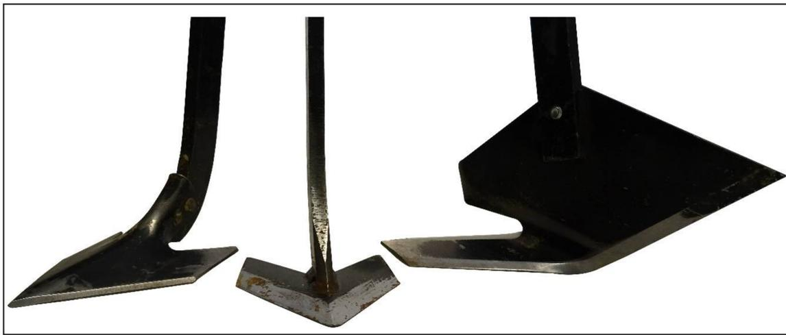
**Figure 2.** Group image of the three cultivation sweeps used in this study. From left to right: goosefoot sweep, no-till sweep and down-cut side knife. The depicted sweeps were adjusted to a row spacing of 150 mm.
