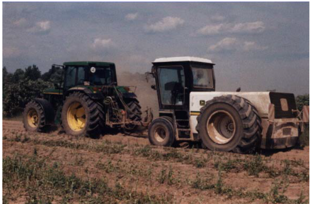
Figure 6. John Deere 6600 tractor and Dyna-Cart dynamometer vehicle.
