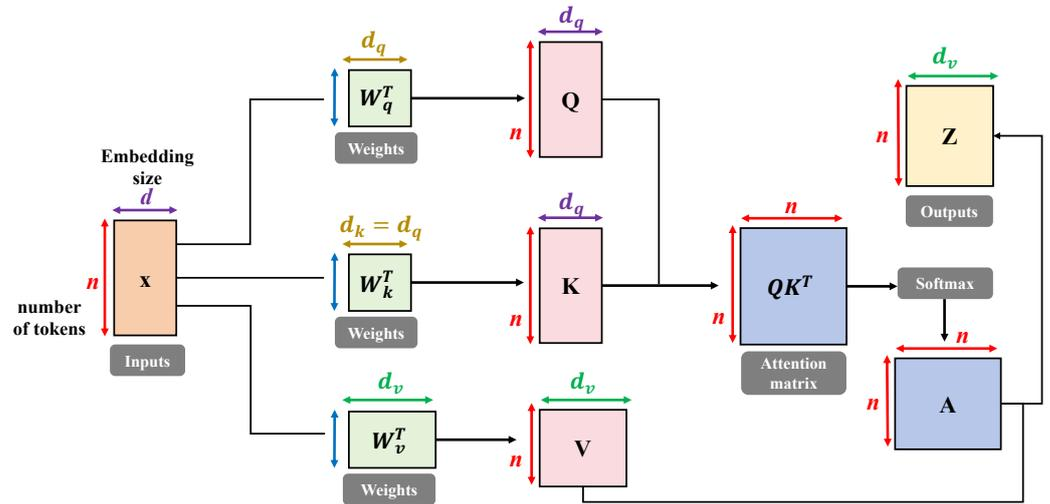
**Figure 5.** Detailed design diagram of the step attention mechanism, showing the process by which the input sequence is transformed into queries (Q), keys (K), and values (V) through the embedding layer and weight matrices, and how these elements generate the attention matrix (A) through self-attention computation, culminating in the production of the output sequence (Z).
