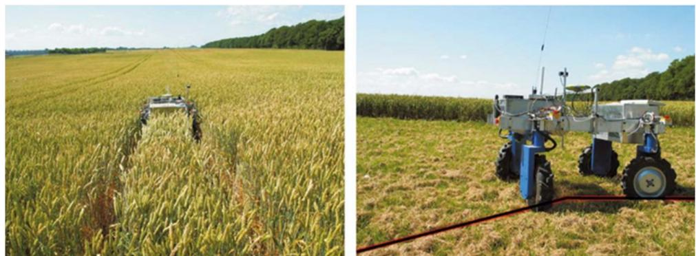
**Figure 3.** Autonomous Weed detector (Reprinted/adapted with permission from [28]).
