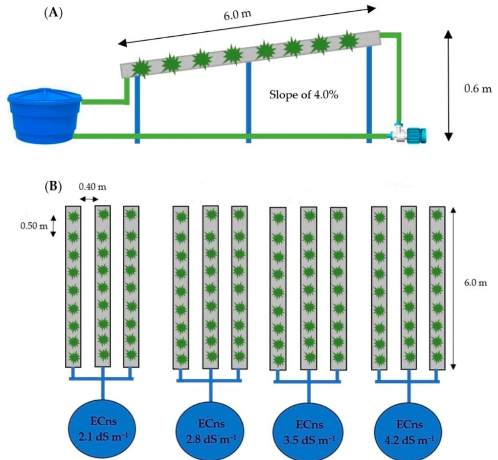
Figure 2. Side (A) and top (B) view details of hydroponic profiles.
