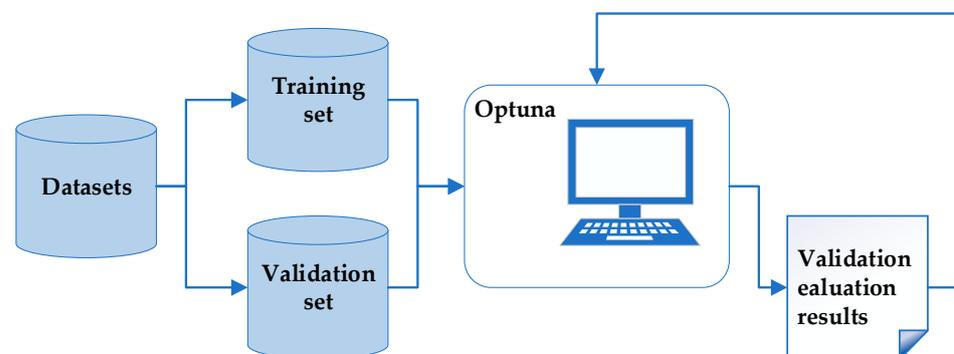
Figure 6. Process of adjusting hyperparameters using optuna.
