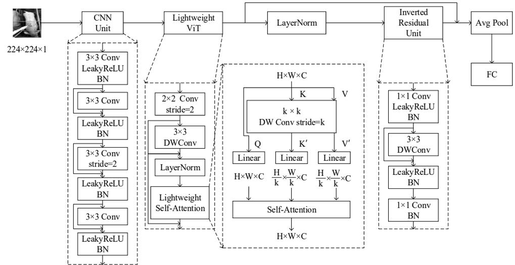
Figure 5. Structure of CNN-ViT feature map measurement model for pregnant sows.
