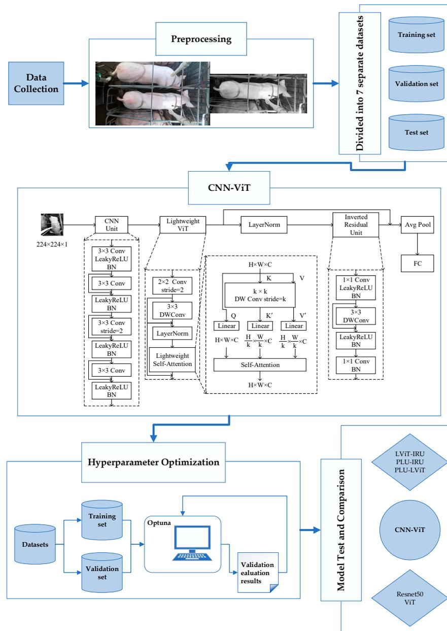
**Figure 1.** CNN-ViT for non-contact measurement of pregnant sows' BF.
