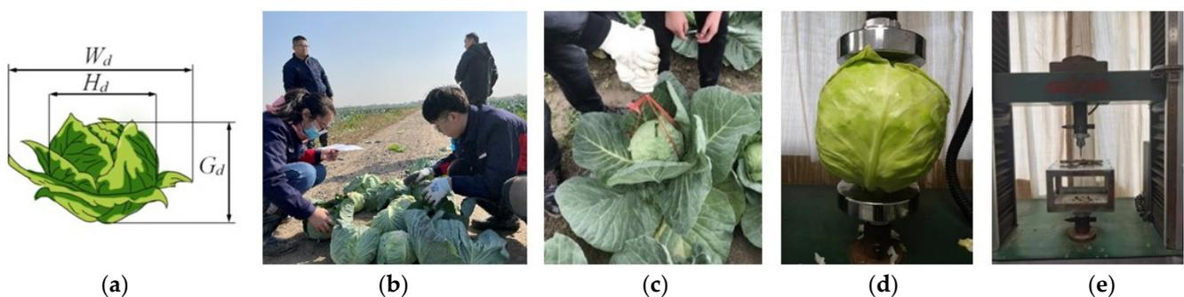
**Figure 1.** Determination of basic physical parameters and harvesting mechanical properties test of cabbage: (a) Physical characteristics acquisition: 1:  $W_d$ : Expansion degree 2:  $H_d$ : transverse diameter 3:  $G_d$ : vertical diameter (b) Physical characteristics acquisition process. (c) Determination of pull-out force. (d) Compression test. (e) Root cutting force test.
