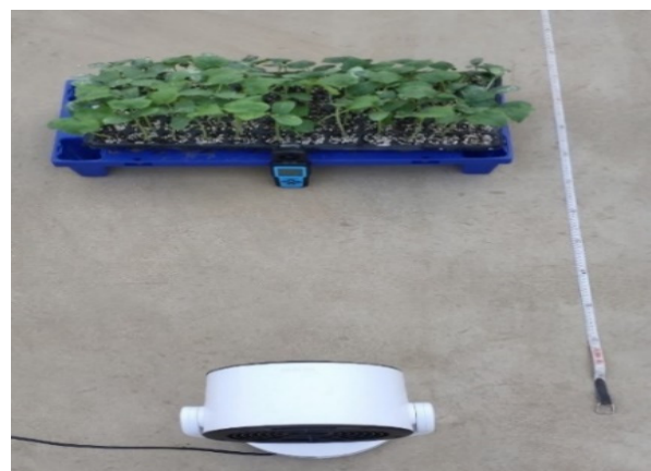
Figure 1. Cucumber seedling airflow disturbance diagram.
