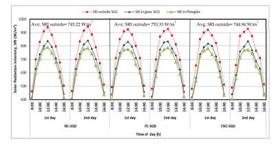
**Figure 5.** Changes in incident SRI in glass and Plexiglas SGDs during typical experimentation days with different drying modes.
