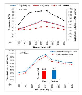
**Figure 6.** Thermal performance of SAH at a air mass flow rate of 0.03 kg/s. (**a**) Variation in solar radiation and temperatures of SAH; (**b**) thermal efficiency of SAH.
