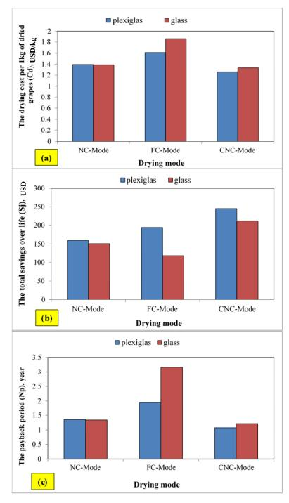
**Figure 11.** Economic assessment of Plexiglas and glass SGDs with different drying modes: (**a**) drying cost per unit of mass of dried grapes, (**b**) total saving cost, (**c**) payback period.
