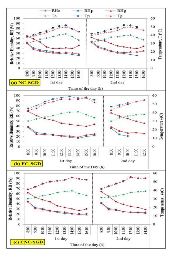
**Figure 7.** Variation in temperatures and relative humidity of air across the glass and Plexiglas SGDs in drying modes (**a**) NC, (**b**) FC ( $m_a = 0.03 \text{ kg/s}$ ) and (**c**) CNC.
