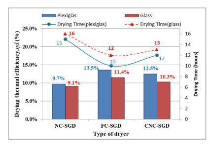
**Figure 9.** The overall drying thermal efficiency and drying time of the Plexiglas and glass SGDs with different drying modes.
