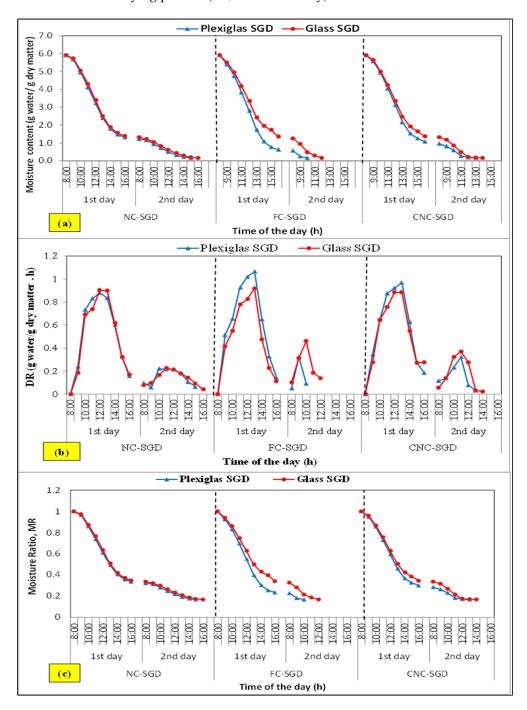
**Figure 8.** Drying behavior of the Plexiglas and glass SGD with different drying modes: (**a**) moisture content, (**b**) drying rate, (**c**) moisture ratio.
