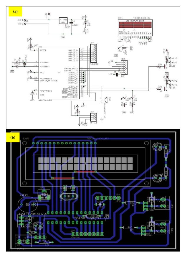
Figure 3. Views of: (a) electronic circuit, (b) the motherboard of ACU.
