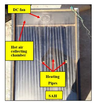
Figure 2. Photograph of SAH used for forced convection drying mode.
