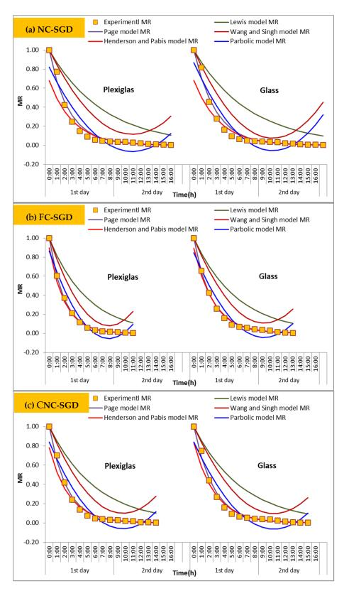
**Figure 10.** The variation in the experimental and predicted MR versus the drying time using glass and Plexiglas SGDs with the different drying modes.
