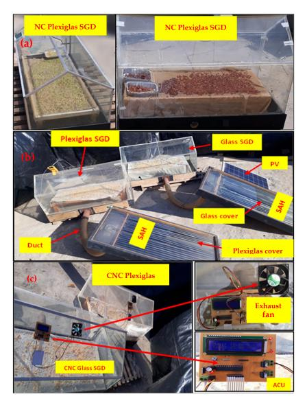
**Figure 4.** The designs of SGD for drying grapes: (**a**) natural convection (NC) mode, (**b**) forced convection (FC) mode, (**c**) controlled natural convection (CNC) mode (new mode).
