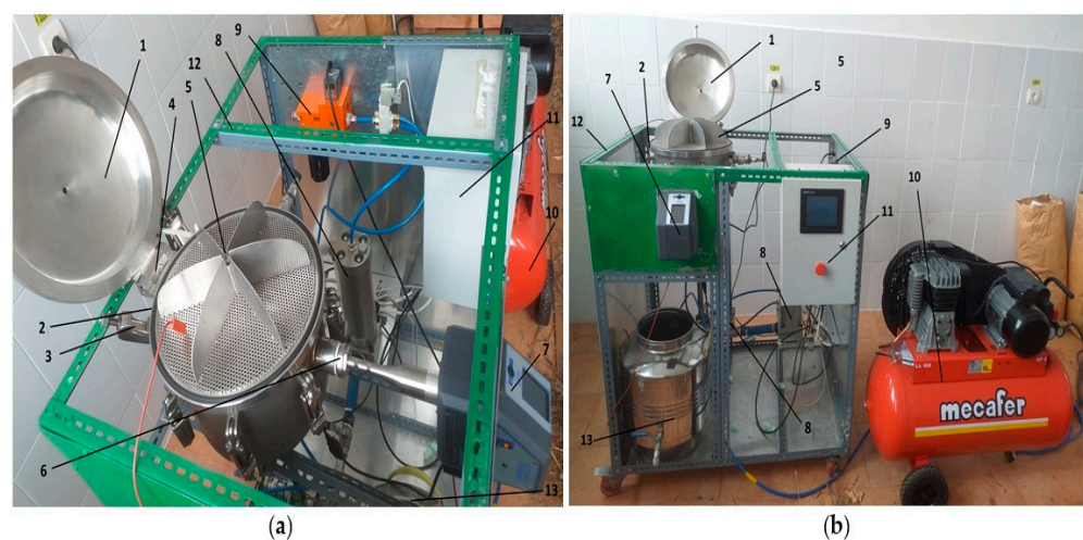
Figure 5. The final design of the pilot equipment used for the extraction of bioactive substances, using a hybrid ultrasound and high-pressure technology: (a) Experimental Extraction Pilot top view, (b) Experimental Extraction Pilot side view.
