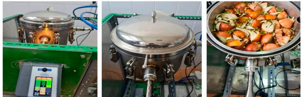
Figure 8. The experimental operation for the ultrasonic extraction mode.
