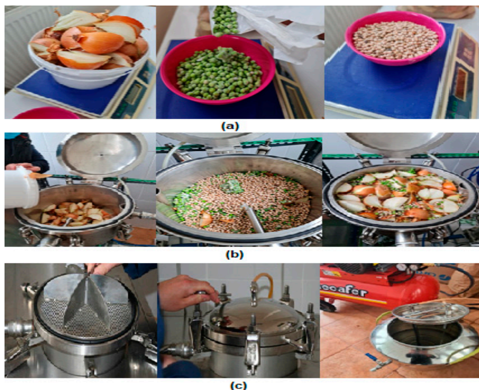
Figure 7. Description of the working method for the production of bioactive compounds: (a) weighing and shredding of the raw material, (b) adding the materials and the solvent to the extraction vessel, and (c) preparing the extraction and the expansion vessels.
