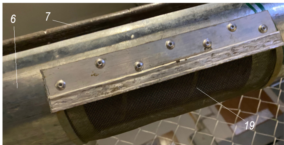
Figure 5. Separating mesh is mounted on the movable in the axial direction of the casing of the telescopic screw conveyor: 6—casing part movable in axial direction; 7—guides; 19—separating mesh.
