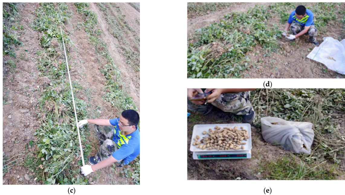
Figure 4. Field experiment flow of peanut digger-inverter: (a) The process of field experiment of peanut digger-inverter. (b) The effect of peanut digger-inverter after field operation. (c) Random 3 m sampling of a stroke after peanut operation. (d) The sampled peanuts were picked manually. (e) The buried pod, fallen pod, and total pod weight of peanuts shall be weighed after operation.
