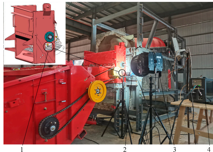
Figure 4. Conveying performance experiment site. 1. Observation window; 2. High-speed digital camera; 3. Light source; 4. Computer.
