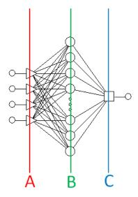
**Figure 3.** Structure of a radial basis function (RBF) with 1 input layer, 1 output layer, and 1 radial hidden layer: A—input layer, B—hidden layer, C—output layer.
