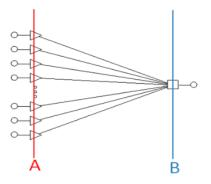
Figure 1. Structure of a linear network with single output. A—input layer and B—output layer.
