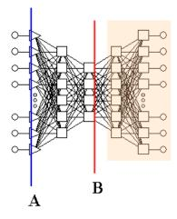
**Figure 4.** A neural auto-associative network implementing a nonlinear PCA transformation: A—input layer of the 5-layer auto-associative network; B—hidden layer of the 5-layer auto-associative network (compressing in a non-inear manner).
