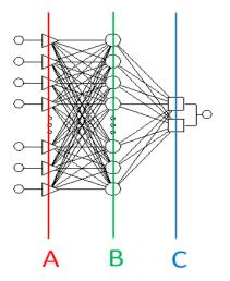
**Figure 6.** Probabilistic neural network (PNN) with 1 input layer, 1 output layer, and 1 radial hidden layer: A—input layer, number of neurons equal to the number of features; B—hidden layer built of radial neurons also called the pattern layer, the number of neurons is equal to the number of learning instances; C—output layer built of linear classifying neurons (summation layer), the number of neurons is equal to the number of classes.
