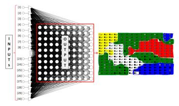
**Figure 5.** An example of the structure of a Kohonen-type neural network applied as a colour (classificator) separator.
