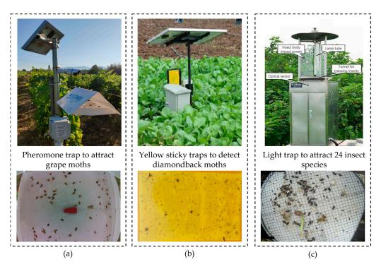
**Figure 1.** Devices installed in the field to collect images of traps and the respective images collected. (a) Pheromone trap in a vineyard to attract grape moths provided by [22]; (b) yellow sticky traps installed to detect diamondback moths adapted from [23]; (c) light trap to attract 24 major pest classes specified by the Chinese Ministry of Agriculture. Images adapted from the dataset Pest24 [24].
