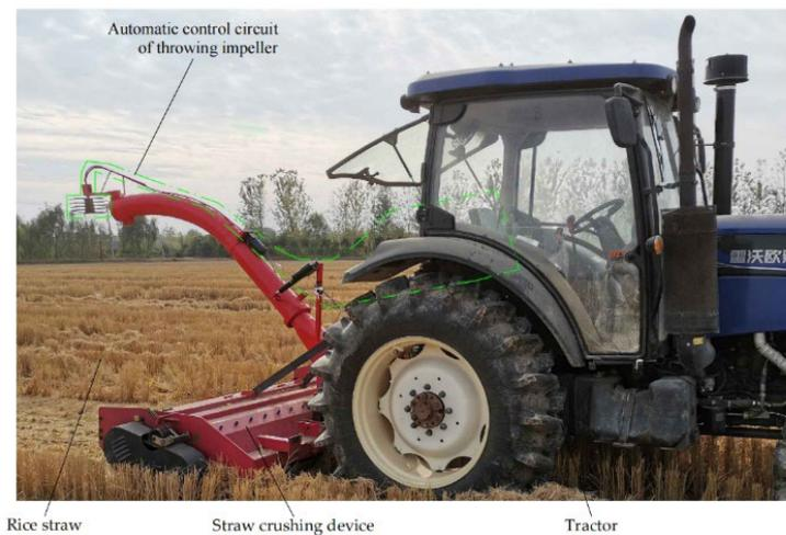
Figure 1. Overall structure of test bed.
