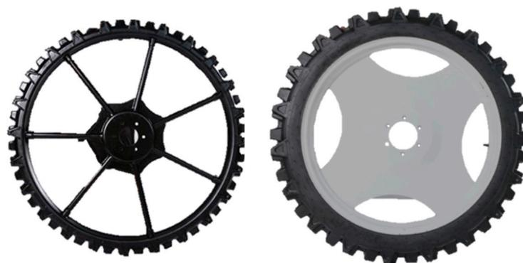
**Figure 6.** Solid rubber tires (left) and pneumatic rubber tires (right).
