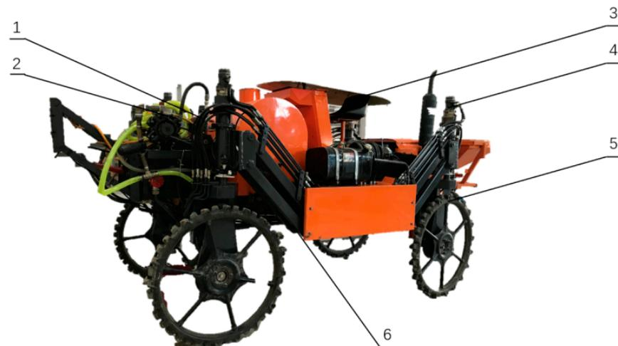
**Figure 1.** Chassis structure diagram: 1—hydraulic system; 2—engine; 3—operating table; 4—outrigger mechanism; 5—wheels; 6—main frame.
