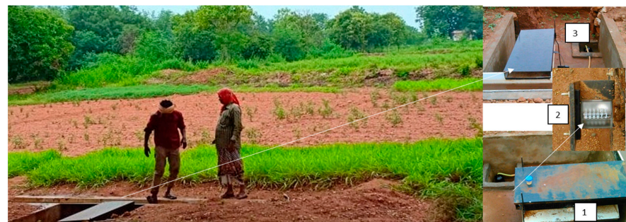
1. Tipping bucket; 2. Magnetic counter; 3. Sample collection point
