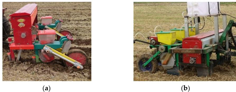
**Figure 2.** Two types of fertilization seeder. (a) Seeder with strip fertilization; (b) seeder with hole fertilization.
