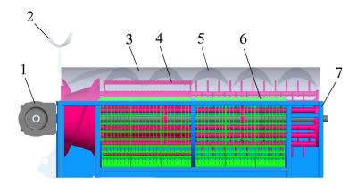
**Figure 4.** Switching diagram of a combination of decide granular device structure: (1) Enter the gearbox of the drum power in the drum. (2) Removing the barrel with the barrel. (3) Persia roller lid. (4) Combined moldy granular drum. (5) Grass guide. (6) Narrow grille concave board. (7) Welding in a departure drum.
