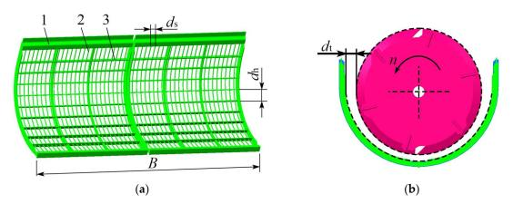
**Figure 7.** Schematic diagram of the structure of the narrow grid recess: (a) Concave plate size. (b) Concave plate-clad corners. (1) Narrow grating concave sieve. (2) Grating bars. (3) Horizontal spacer. Note:  $d_s$  is the spacing between the grating bars in mm;  $d_h$  is the spacing between the horizontal dividers in mm;  $d_t$  is the gap between the concave plates in mm.
