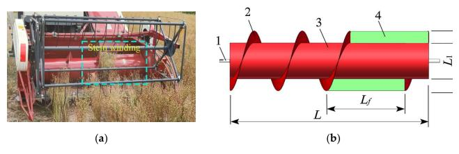
**Figure 3.** Diagram of the churn winding and anti-winding device: (a) Churning dragon wrap. (b) Diagram of the anti-tangle device. (1) Churning dragon wrap. (2) Diagram of the anti-tangle device. (3) Stirrer. (4) Anti-winding plate. Note: L is the length of the churn in mm.  $L_f$  is the length of the anti-winding plate in mm.  $L_1$  is the diameter of the churn in mm.  $L_2$  is the long shaft of the anti-winding churn in mm.
