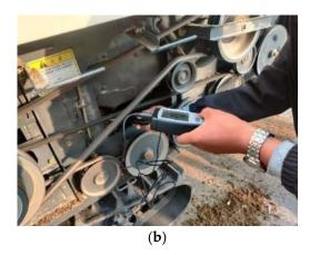
**Figure 11.** Determination of threshing drum speed and centrifugal fan airspeed on the prototype: (a) Threshing drum speed determination. (b) Centrifugal fan outlet air velocity determination.
