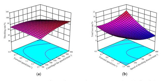
**Figure 13.** Influence of interaction factors on response values: (a) Effect of advancing speed and centrifugal fan speed on decontamination rate. (b) Effect of advancing speed and threshing drum speed on total loss rate.
