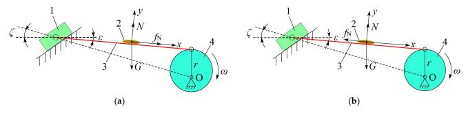
**Figure 9.** Kinematic model of a vibrating screen: (a) Slip-on detachment. (b) Slippage of debris. (1) limit slider. (2) Flaxseed grain. (3) Sieve surface. (4) Eccentric wheel. Note: G is the gravity of the flaxseed grain, N; N is the support force on the flaxseed grain, N;  $F_n$  is the friction force on the sieve surface on the flaxseed grain, N;  $\omega$  is the angular speed of the eccentric bearing in rad·s<sup>-1</sup>.
