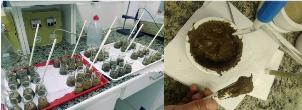
Figure S2. Different soil samples in triplicate are checked for its PH (left image), and for soil type by Arany method.
