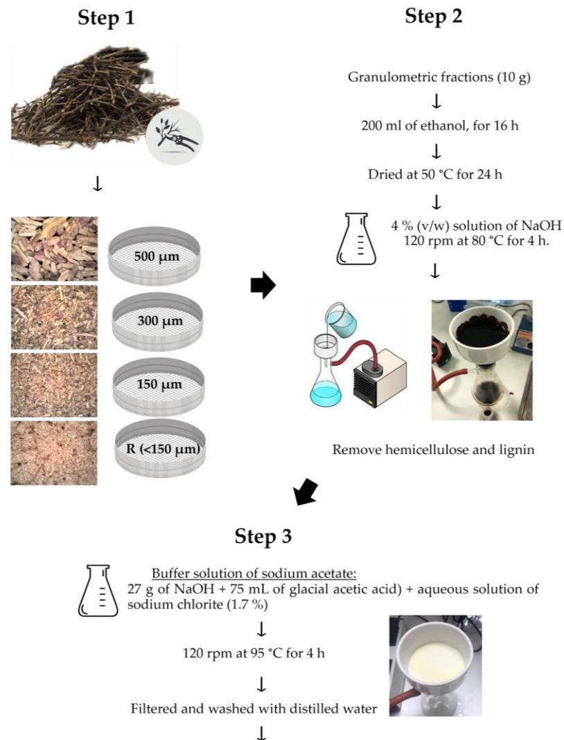
**Figure 1.** Schematic representation of the treatment steps of vine prunings: step 1—granulometric fractions; step 2—treatment; step 3—bleaching.
