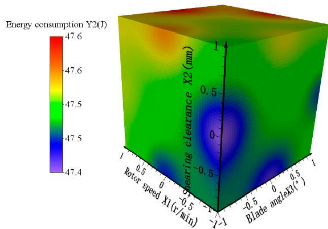
**Figure 15.** Four-dimensional rendering graph illustrating the influence of the cutter shaft speed, cutting clearance, and cutter edge angle on the energy consumption of straw crushing.
