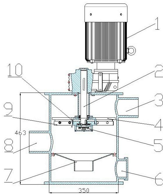
**Figure 1.** Structure chart of the crushing and impurity removal device. (1) Adjustable-speed motor, (2) transmission shaft, (3) outlet, (4) cutter head, (5) cross rotary cutter group, (6) impurities outlet, (7) funnel, (8) inlet, (9) cross tool holder, (10) blade.
