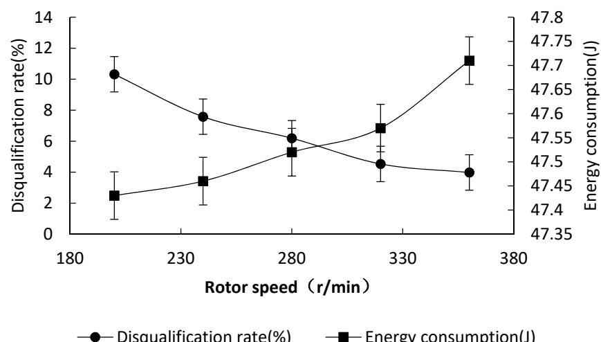
**Figure 10.** Experimental results of the influence of the cutter shaft rotor speed on the qualification rate and energy consumption of straw crushing.
