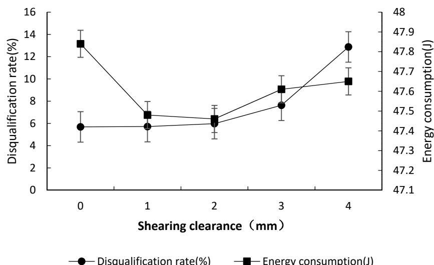
**Figure 11.** Experimental results of the influence of the cutting clearance on the qualification rate and energy consumption of straw crushing.
