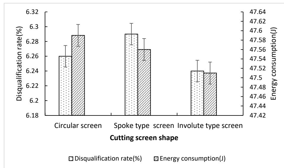
**Figure 9.** Experimental results of the influence of the cutter head cutting screen shape on the qualification rate and energy consumption of straw crushing.
