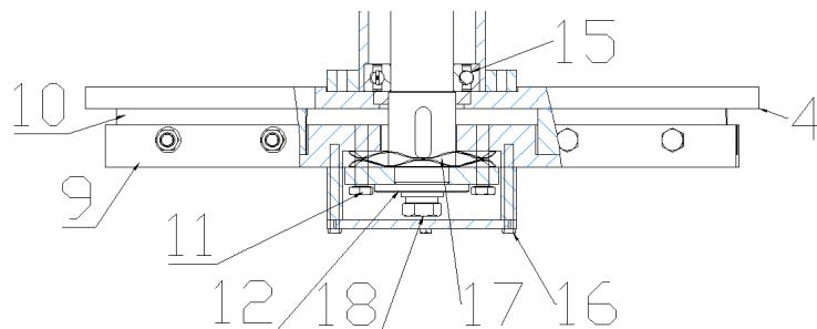
**Figure 3.** Cross rotary cutter group. (4) cutter head, (9) cross tool holder, (10) blade, (11) Bolt guide, (12) shaft end washer, (15) bearing, (16) fixed bolt, (17) multilayer wave spring, (18) shaft end bolts.
