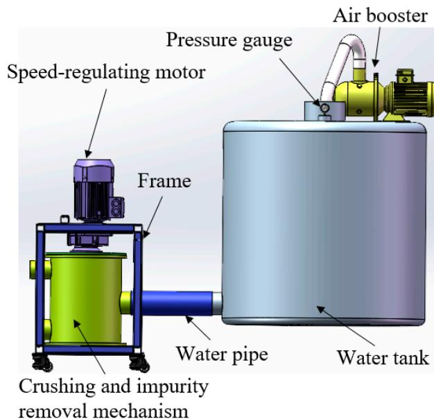
**Figure 6.** Schematic of the test platform.
