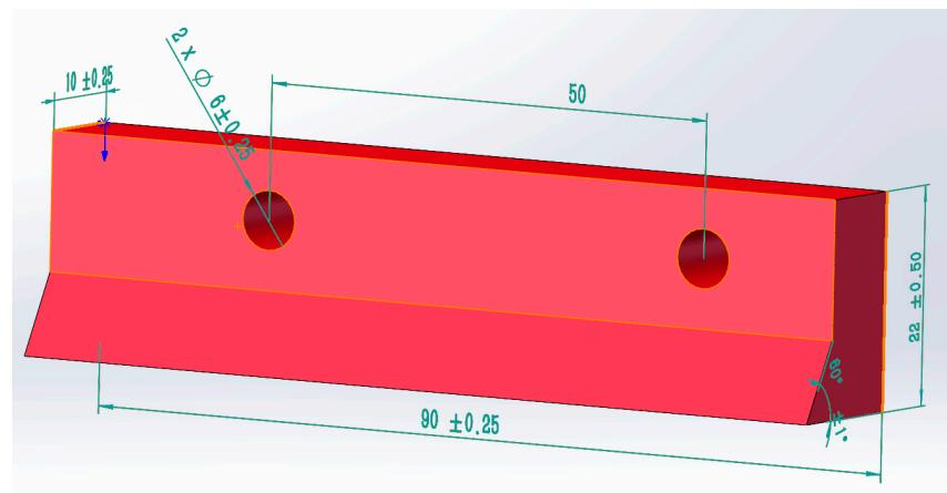
**Figure 13.** Schematic of the blade.
