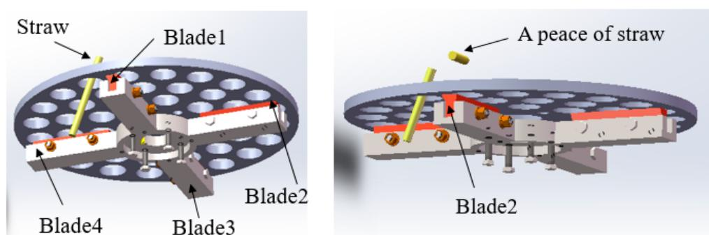
**Figure 4.** Cutting process of straw.
