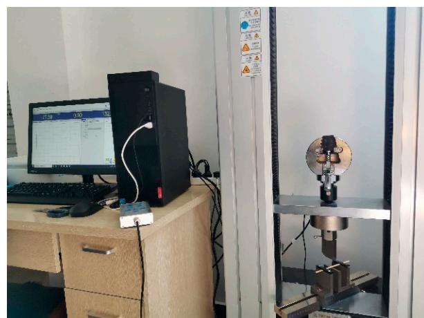
**Figure 2.** Straw shear force test.
