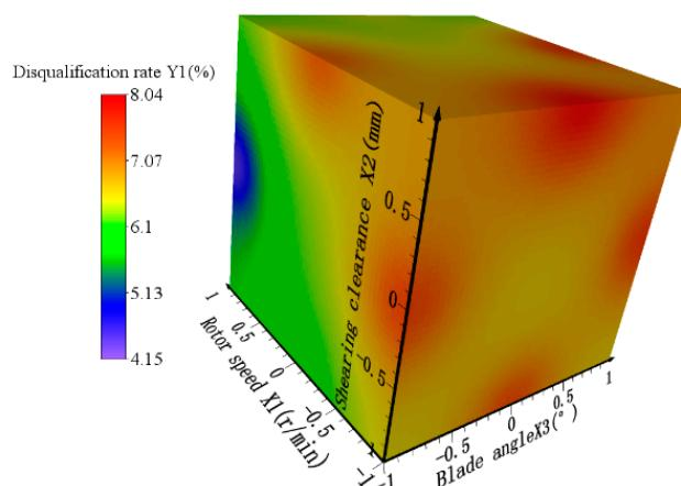
**Figure 14.** Four-dimensional rendering graph illustrating the influence of the cutter shaft speed, cutting clearance, and cutter edge angle on the disqualification rate.
