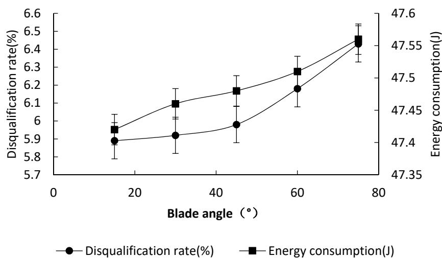
**Figure 12.** Experimental results of the influence of the cutter edge angle on the qualification rate and energy consumption of straw crushing.
