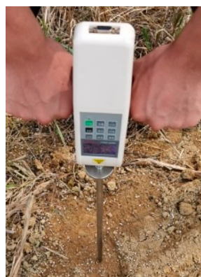
Figure 2. Portable electronic soil penetration resistance tester.
