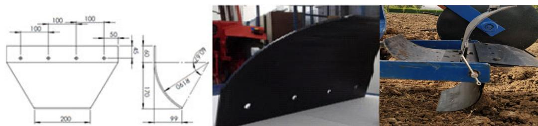
**Figure 10.** Design and construction of a curved optimized blade equipped with the furrow compartmenting system rotor.
