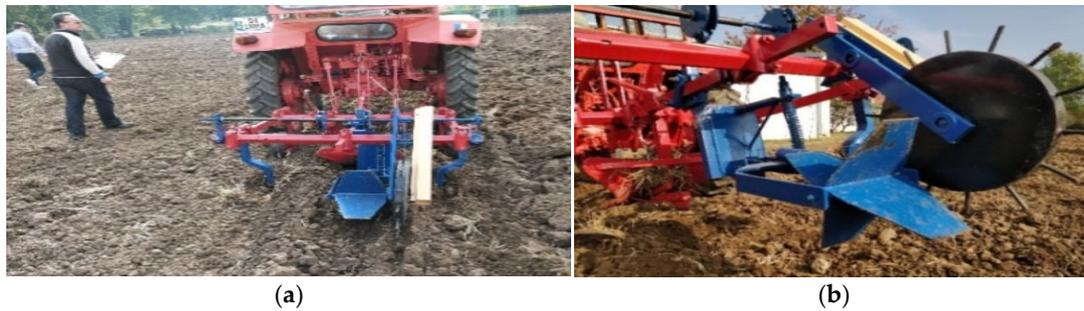
**Figure 15.** Testing the furrow diking system equipped with the standard rotor blades. (a) Testing the equipment performance on difficult soils. (b) Evaluation of the equipment wear during testing.
