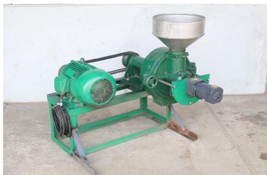
**Figure 9.** Rice straw fiber crusher test prototype.
