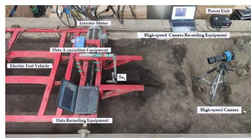
Figure 11.  $Su_3$  experiment of soil bin.
