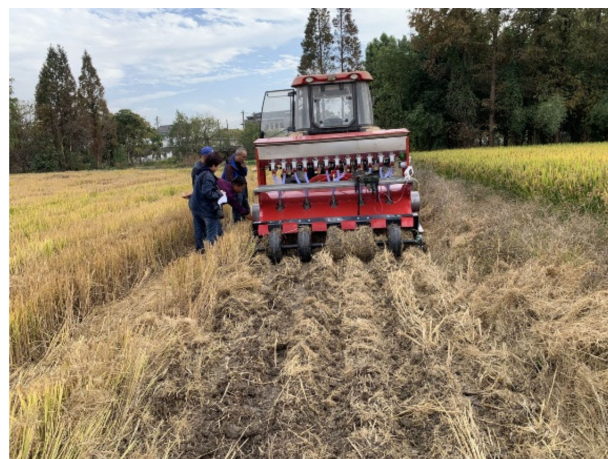
Figure 4. Existing problems with straw back throwing and strip laying.
