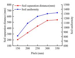
**Figure 11.** Relationship curves between pitch and *D*<sub>W</sub>, *E*.
