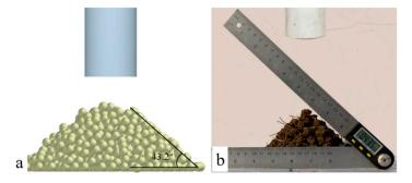
Figure 5. (a,b) Angle of repose experiment of soil.
