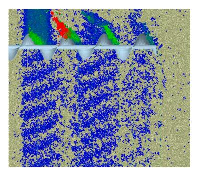
Figure 15. Simulation results after optimizing parameters of spiral soil separating device.
