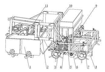
**Figure 1.** General structure of compound planter. 1. Biaxial rotary tillage mechanism. 2. Connecting rod. 3. press grooving roller. 4. Seeder. 5. Seed box. 6. Spiral soil separating mechanism. 7. Repress roller. 8. Ditcher. 9. Steering box. 10. Transmission shaft. 11. Intermediate transmission box.
