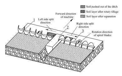
Figure 2. Working process of SSSM. 1. Left spiral blades. 2. Ditching. 3. Right spiral blades.
