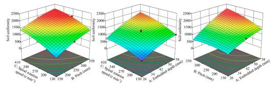
Figure 14. Response surface analysis of the relationship between test factors and soil uniformity.
