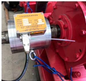
**Figure 6.** Installation of torque sensor.
