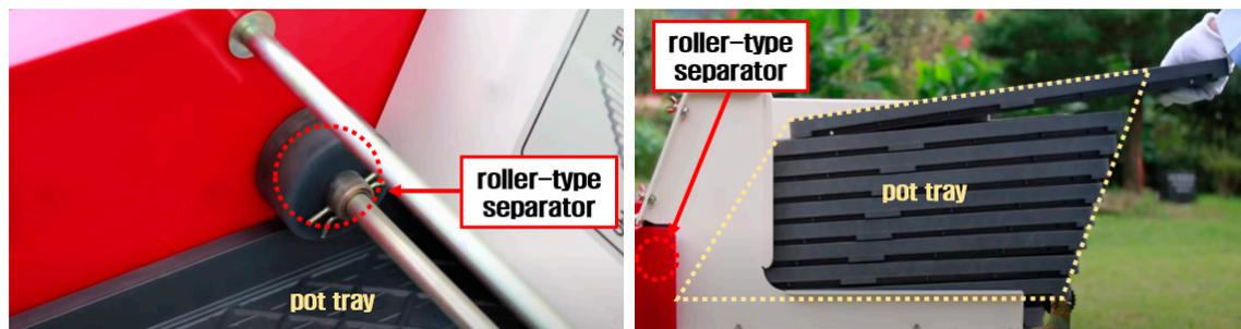
Figure 6. View of the pot autofeeding device with a roller-type separator applied.
