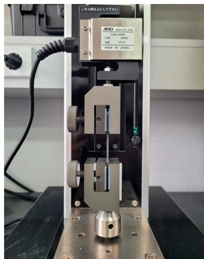
Figure 7. View of the universal testing machine used.
