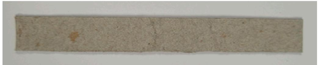
**(a)** biodegradable pot tray
