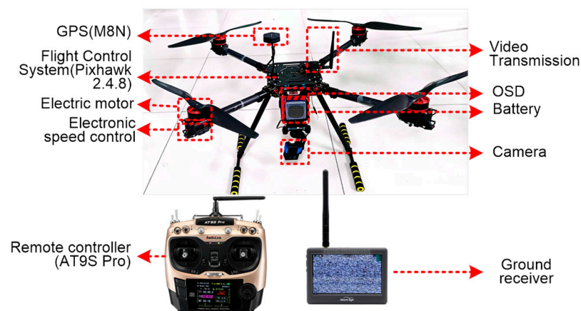
Figure 5. Assembled FPCS and part assignment.
